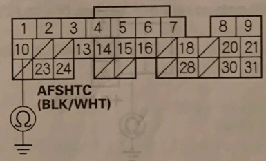
Wire side of female terminals
