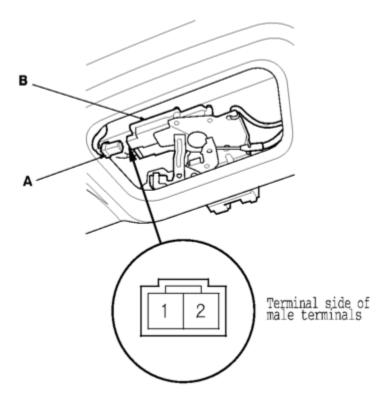
Check actuator operation by connecting power and ground according to the table. To prevent damage to the actuator, apply battery voltage only momentarily.
