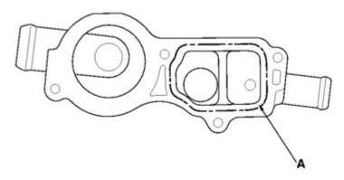
Install the rubber seal (A) on the thermostat (B),
