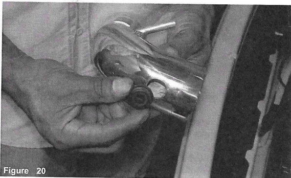
Figure 18 The harness clip is compressed and push through the fender in order to free the electrical harness.
