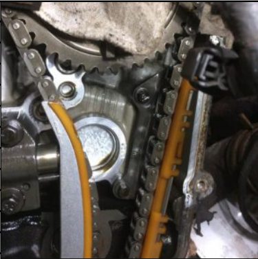
The left side of the timing chain is not riding on the guide, it's down in the guide.
