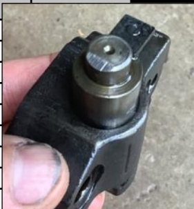
The timing chain tensioner is clearly worn on one side.
