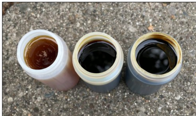
Left: Virgin oil. Center: oil run 5 minutes. Right: oil run several thousand miles.
