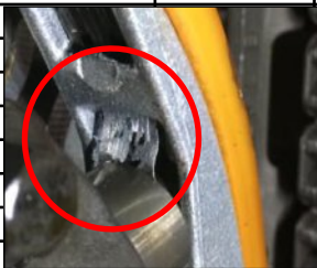
The left side of the timing chain is not riding on the guide, it's down in the guide.
