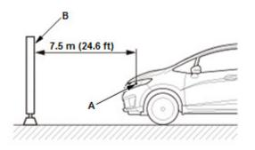
Park the vehicle so that the center mark of the **headlight** (A) is 7.5 m (24.6 ft) away from a wall or screen (B).
