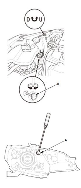
If adjustment is necessary, open the hood and adjust the **headlights** to local requirements by turning the adjuster (A).
