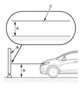
Measure the height of the headlight's center mark (A), then on the wall or screen (B), mark the same height of the headlights with masking tape in a straight horizontal line (C).
