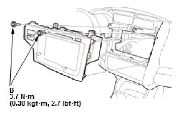
1. Install the audio-navigation unit in the reverse order of removal.
