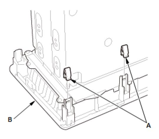
2. Remove the clips (A) from the audio pa (B).
