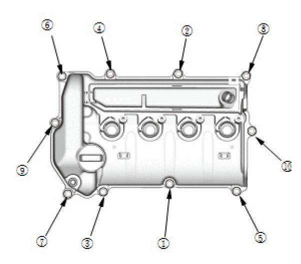
7. Tighten the bolts in two steps. In the fir step torque bolts, in sequence, to 7 N·r kgf·m, 5 lbf·ft).
