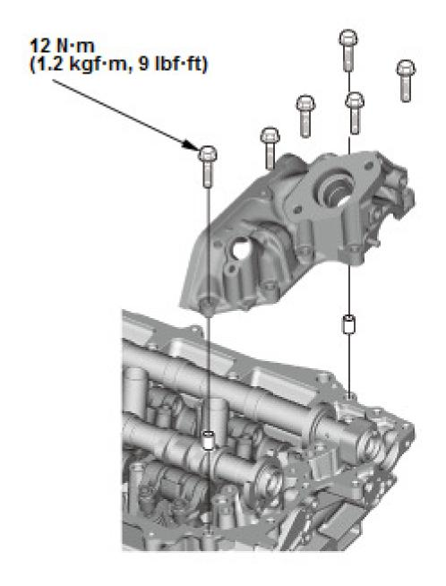
3. Install the high pressure fuel pump cov NOTE:
