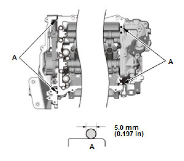
5. Apply liquid gasket, (P/N 08717-0004, 08718-0003, or 08718-0009) on the chacase and the No. 5 rocker shaft holder mating areas (A). Install the component within 5 minutes of applying the liquid gasket.
