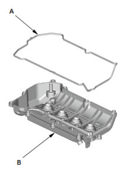
Thoroughly clean the head cover gaske and the groove of the cylinder head cov (B).
