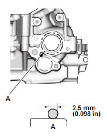
4. Remove all of the old liquid gasket from cylinder head, the high pressure fuel processor, and the cam holder cover.
