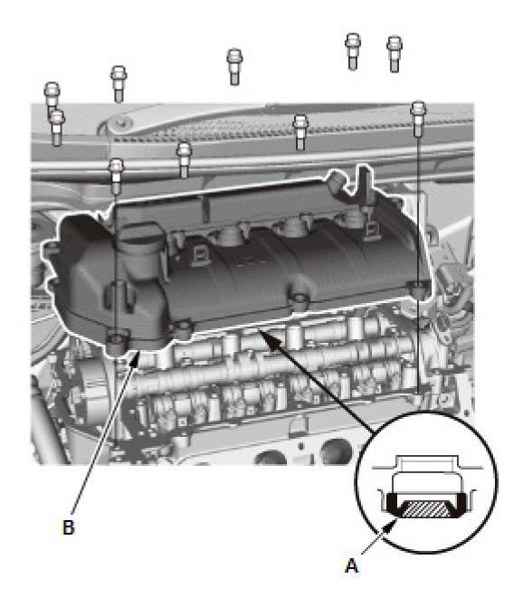
6. Apply new engine oil to the rip of the splug seals (A). Place the cylinder head(B) on the cylinder head, then slide the slightly back and forth to seat the head
