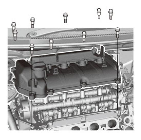
7. Remove the cylinder head cover.
