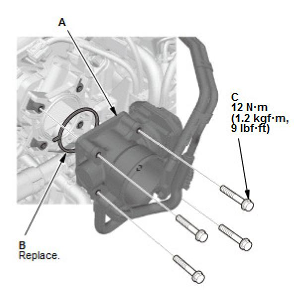
1. Install the throttle body (A) with a new (
