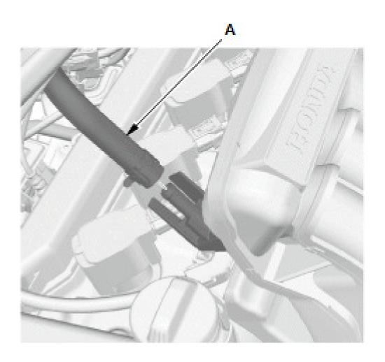
Disconnect the brake booster vacuum ł(A).
