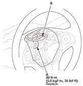
6. Install a new steering wheel bolt (A), and tighten it to the specified torque.
