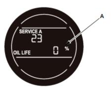
5. If the indicated maintenance is not done, the engine oil life indicator shows a negative distance traveled, for example "-10" on the display. If the negative distance traveled is between 0 and -9, the indicator is displayed for only a few seconds when the vehicle in the ON mode. The negative distance traveled remains displayed after the vehicle is driven more than 10 miles (for USA models) or 10 km (for Canada models) after 0 % oil life is reached, and the display cannot be canceled.
