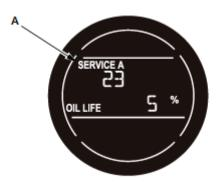
4. When the vehicle in the ON mode, and the remaining engine oil life is 0 %, the engine oil life indicator (A) blinks. Pressing the Select/Reset knob cancels the display, but the Maintenance Minder indicator stays on.
