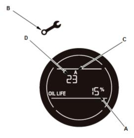
3. When the vehicle in the ON mode, and the remaining engine oil life is 5 % to 1 %, the message "SERVICE" (A) is displayed along with engine oil life and the same maintenance item code(s).
