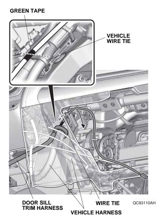
21. Route the door sill trim harness as shown. Then secure it to the steering hanger beam with three wire ties.
