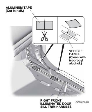
49. Using scissors, cut the aluminum tape in half. Secure the right front illuminated door sill trim harness to the vehicle panel with aluminum tape. 50. Secure the right front illuminated door sill trim harness to the vehicle harness with two wire ties.
