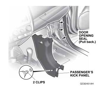
6. Pull back the door opening seal, and remove the driver's front door sill trim.
