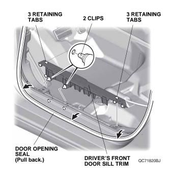
7. Pull back the door opening seal, and remove the driver's kick panel.
