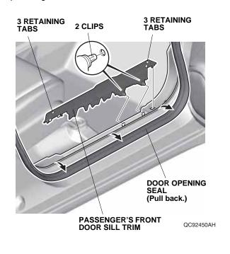
5. Pull back the door opening seal, and remove the passenger's kick panel.
