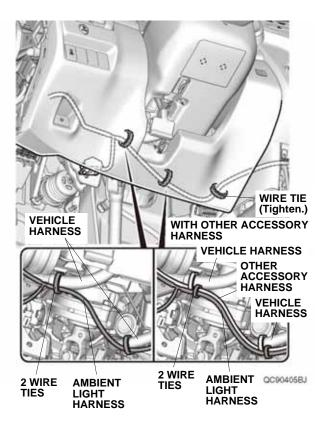
18. Secure the ambient light harness to the vehicle harness with one wire tie.
