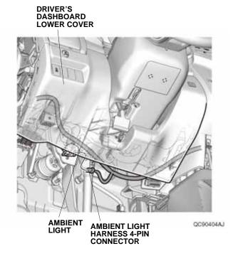
17. Secure the ambient light harness to the vehicle harness with two wire ties. If the other accessory harness is already secured to the vehicle harness, secure the ambient light harness to the other accessory harness with two wire ties. Tighten the wire tie.
