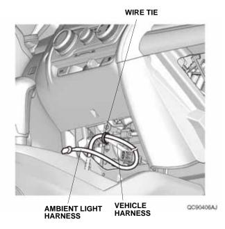
19. Route the ambient light harness as shown. Secure the ambient light harness to the vehicle harness with three wire ties.
