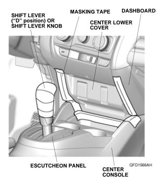
7. Remove the center lower cover, and unplug the vehicle connectors.
