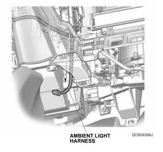
21. Install the ambient light on the passenger's under cover with one self-tapping screw.
