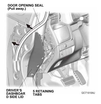
5. Remove the driver's dashboard lower cover, and unplug the vehicle connectors.
